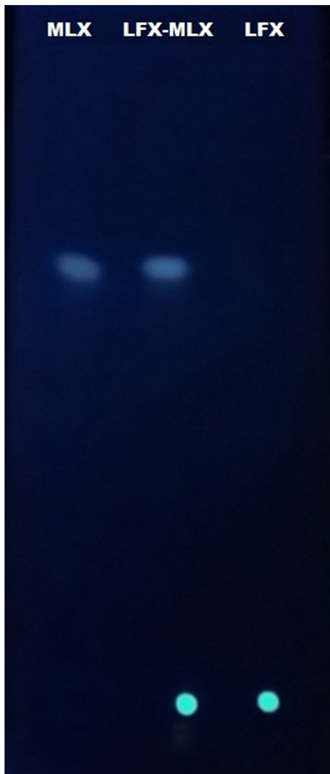
Fig. 4. MLX, LFX-MLX, and LFX spots on the plate; wavelength 366 nm; no.1 mobile phase
