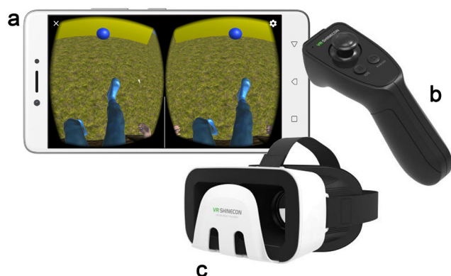
Fig. 4. IVR equipment: a. Lenovo Vibe K6; b. VR Shinecon blue-tooth gamepad; c. 3D VR Shinecon glasses for mobile phone
