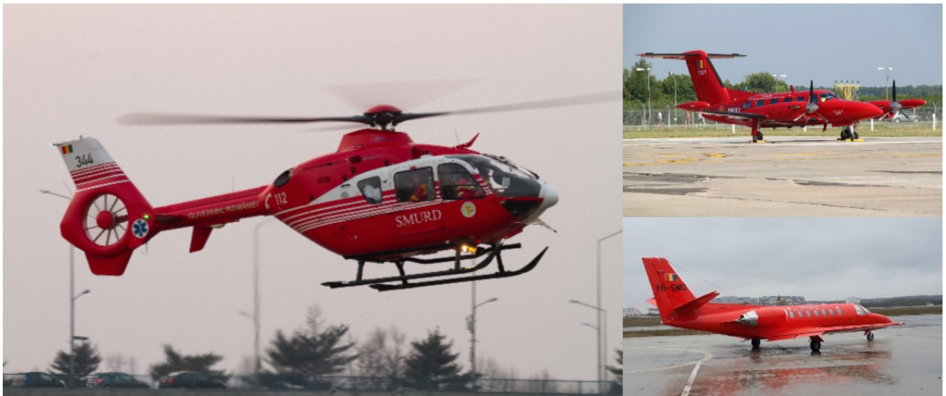
Fig. 1. Aircrafts of the SMURD organization, at left is the Airbus helicopters H-135 helicopter, at the top-right is the Piper PA-42 Cheyenne, and the Cessna Citation V is at bottom-right.
